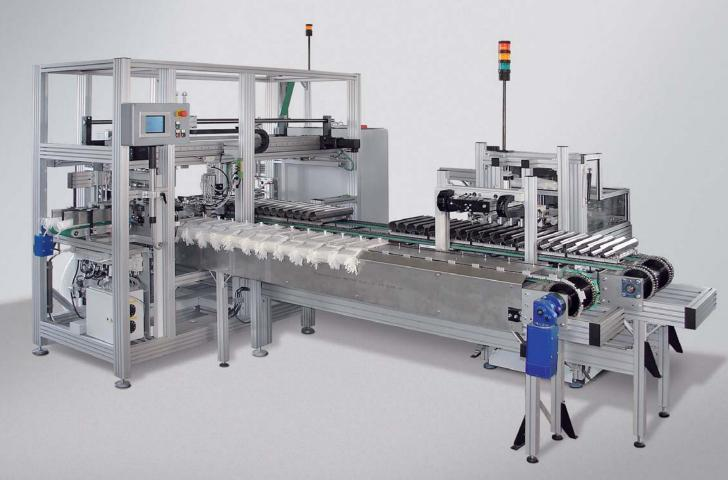
Fully automated bagging and packaging machine for cotton pads and related products
