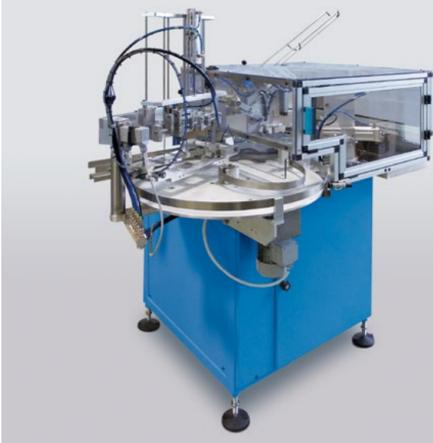
RB-30A is a fully automatic cotton swab packaging machine for round boxes to be combined with a Falu cotton swab machine.
