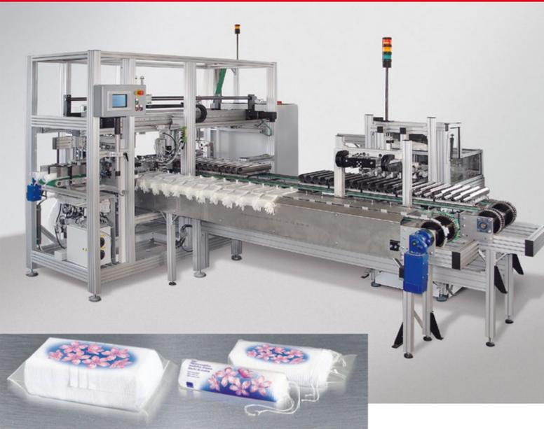
FALU RB-2 is a fully automated bagging and packaging machine for cotton pads and related products.
